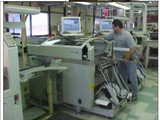
LEFT: Dave Rohan, Production Engineer and a 9th year Raven employee, holds a stencil that begins the process to make the Printed Circuit Boards (PCB). CENTER: Kelly Stern, SMT Technician and an 8th year employee, enters the correct information into the computer to create the various PCBs, including the rate of production. RIGHT: Stern is seen adjusting the automated, Pic & Place Machine. UPPER LEFT: Upclose photo of PCBs made at RI.
