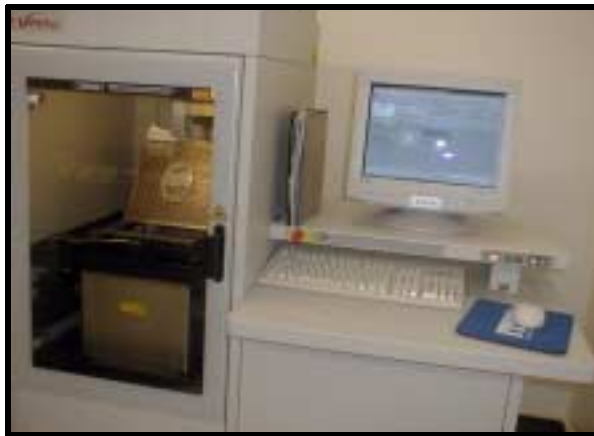
ABOVE: The Viper machine shows the finished master part. RIGHT: The master part is resting on the platform. Resin drippings can be seen on the panel. (Step 2)
