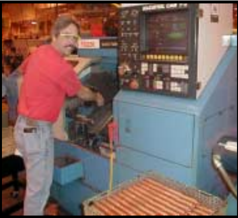
ABOVE: Jeff Dargatz, a CNC Machinist is working by a machine with a Controller. This has the program that tells machine how to make the torch parts from mostly brass.
