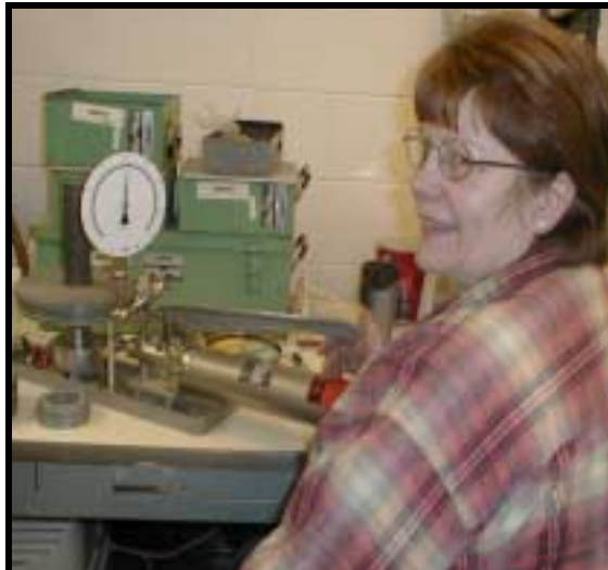
LEFT: Carolyn DesLauriers, a Manufacture Technician is working the Quality gauge tester to see if the gauge is properly functioning. ABOVE: A close up shot of the pressure gauge tester showing the scale calibrating 0-400 pounds of pressure.
