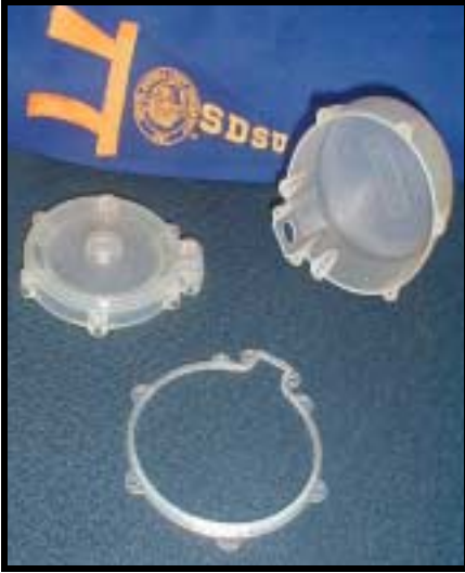
LEFT: GPRPC finished master mold for Raven Industries. ABOVE: Finished product including a urethane elastic gasket made by GPRPC staff for Raven Industries.
