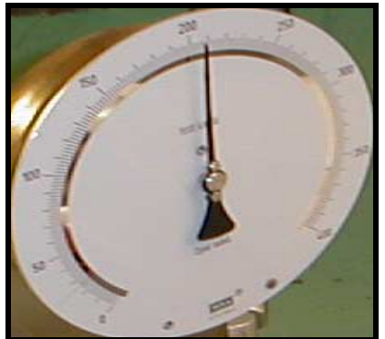
LEFT: Carolyn DesLauriers, a Manufacture Technician is working the Quality gauge tester to see if the gauge is properly functioning. ABOVE: A close up shot of the pressure gauge tester showing the scale calibrating 0-400 pounds of pressure.
