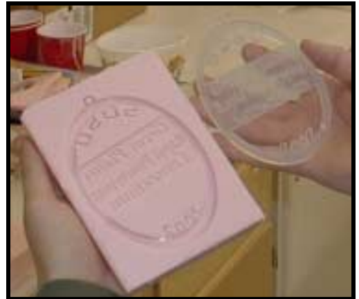
LEFT: Wearing protective gear, Jerry Visser removes the master part from the Viper. ABOVE and RIGHT: The SLA machine makes the master part that is used in making the silicon mold. (Step 3)
