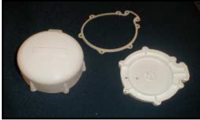
LEFT: GPRPC finished master mold for Raven Industries. ABOVE: Finished product including a urethane elastic gasket made by GPRPC staff for Raven Industries.
