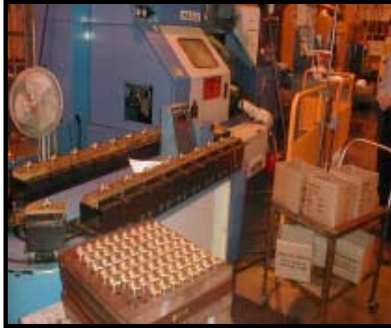
ABOVE: An automated machine is shown machining, forging, milling and drilling to produce heads. The robotic arm is reaching inside the machine for a part. ABOVE RIGHT: A 15-year-old automated machine. RIGHT: Tammy Klose, CNC Operator of Automation Equipment, where it's "quite busy and a lot of hours."
