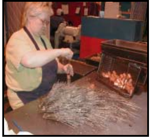
ABOVE LEFT: Michael Greeley, CNC Machinist, holds a drilled part. The background shows one of the old machines. Inset photo: Shows how the old machines drill holes around the perimeter. ABOVE RIGHT: Cindy Helwig, a Wire Technician, demonstrates how wires are insert around the perimeter. These are gel coated so the wires slide easier. “A Technician can do 300 easily per hour,” said Helwig.
