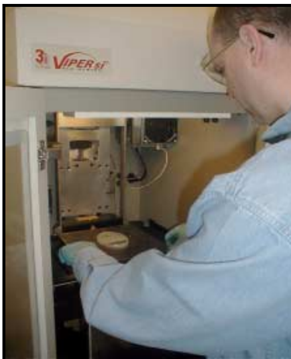
ABOVE: The Viper machine shows the finished master part. RIGHT: The master part is resting on the platform. Resin drippings can be seen on the panel. (Step 2)
